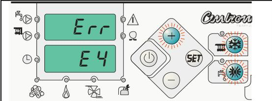
To enable control unit to resume to normal operation, error must be corrected and cancel it on the control unit. Error is cancelled by simultaneous pressing **WINTER** and **SUMMER** buttons and "+" button. If the error cause is not repaired, error cannot be cancelled.
